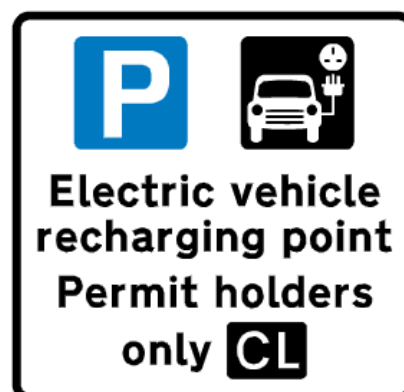
Figure 16: Example signage for chargepoints in CPZs
